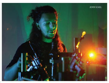
**LUCA TROISE**, a postdoc at the Technical University of Denmark, uses a quantum diamond sensor to measure neural activity in a slice of mouse brain. Magnetic fields from firing neurons affect spins in the sensor, which in turn govern the resulting fluorescence. The project is part of the new Copenhagen Center for Biomedical Quantum Sensing.
