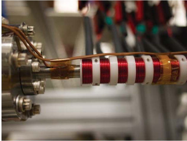
Figure 5.3: Photograph of the hydrogen coilgun coil wound around the slowing chamber. The coils are held in place by Delrin clamps, which are clamped onto the chamber before the coil is wound.
