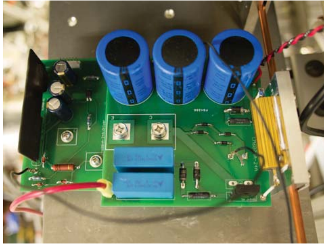
Figure 5.5: Photograph of the hydrogen coilgun coil driver circuit. The board on the right is the circuit which drives the coils, while the board on the left is the circuit which drives the gate of the IGBT.
