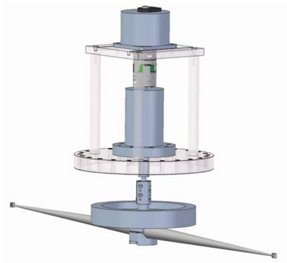
Figure 3.9: A CAD image of the rotor as held by the initial spindle. The spindle is rigidly coupled to the shaft of the ferrofluidic feedthrough. The feedthrough attaches to a 10 – 4.5 inch zero length reducer, which supports the spinning parts, as well as the motor, which is mounted above the feedthrough via a flexible coupling. Figure Courtesy Max Riedel.
