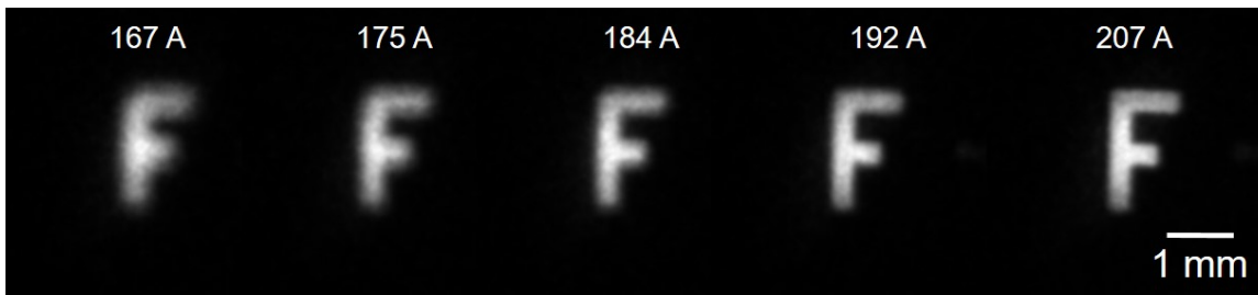
Figure 8.20: Focusing sequence for the F-shaped aperture with the double peak correction field in place. Unlike in Figure 8.11, we present the image right-side up. Image distance is 113 cm.
