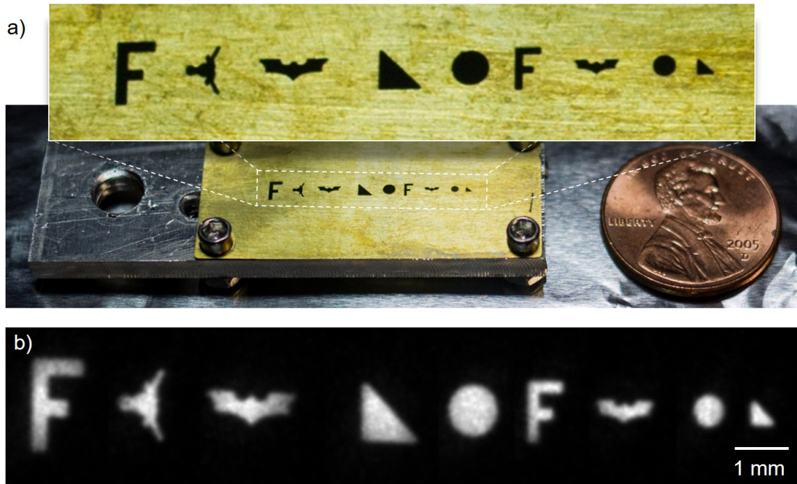
Figure 8.22: (a) Photograph of the slide, for easy reference. (b) Composite image of the slide, again at 113 cm. Though the sizes are matched in this case, the magnification factor is 0.81.
