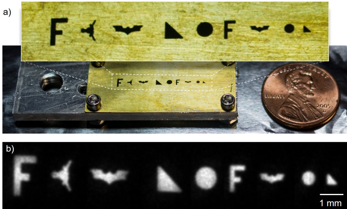
Figure 1.6: A preview of the images we produce using a first-generation prototype of the pulsed electromagnetic hexapole. Our image quality and resolution (along with our choice of shapes, in our opinion) are significantly improved over results from previous hexapole lenses (e.g., Figure 1.5).
