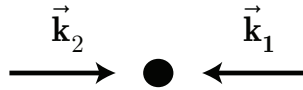
Figure 4.4: Molasses. Two red-detuned near-resonant beams are propagating in the directions \vec{k}_1 and \vec{k}_2 . When the atom moves to the right, it scatters more photons from beam 1, when it moves to the left, it scatters more photons from beam 2. The faster the atom moves, the more it scatters.
