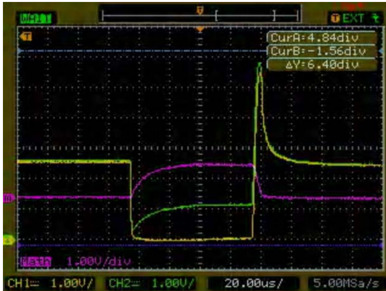
Figure 4.5: This figure shows a typical current evolution in the coil during an 80 \mu\text{s} capacitor discharge measured over the 0.25 \Omega resistor (see figure 4.4) using 1/100 probes. The yellow curve is measured in front of the resistor, the green one after and the pink is the difference, i.e. 1/4 of the current. Although the current drops from 400 A to 0 A within 7 \mu\text{s} the magnetic field remains at about 20 % of its peak value due to Eddy currents and the hysteresis of permendur (see figure 4.7).
