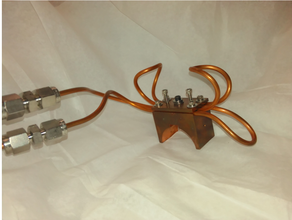
Figure 8.2: Image of the cooling assembly that mounts on top of the beam head. The copper tubing runs across the top of the heat sink four times and it is recessed into grooves for better thermal coupling. The heat sink approximates the shape of the beam head and fits tightly. There is one hole in the side face of the heat sink that allows for mounting of a thermocouple wire to measure the temperature of the top of the beam head, underneath the heat sink.
