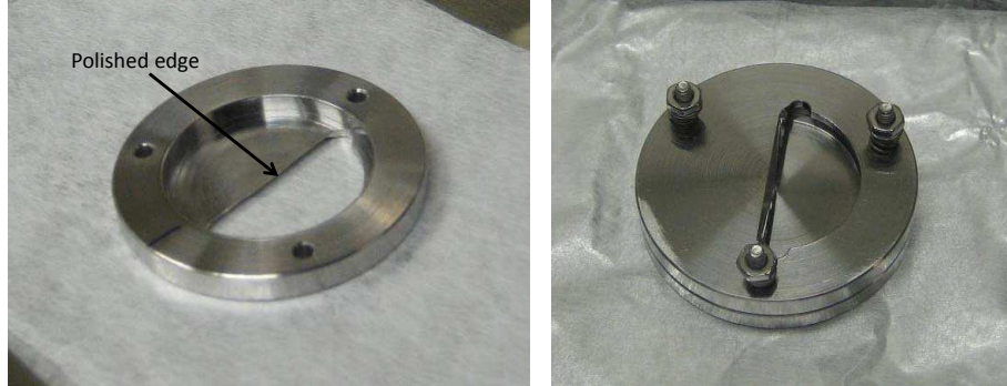
Figure 6.45: Picture of the steel mask used to create the phase plate for the TEM_{01} mode.
