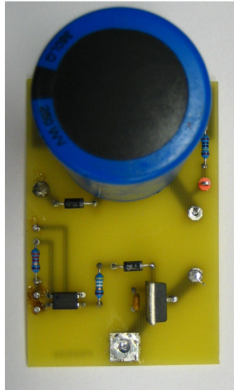
Figure 3.5: A picture of the individual board for each coil. The coil is fired by passing 258 V through 0.34 \Omega total resistance for 100 \mu s .
