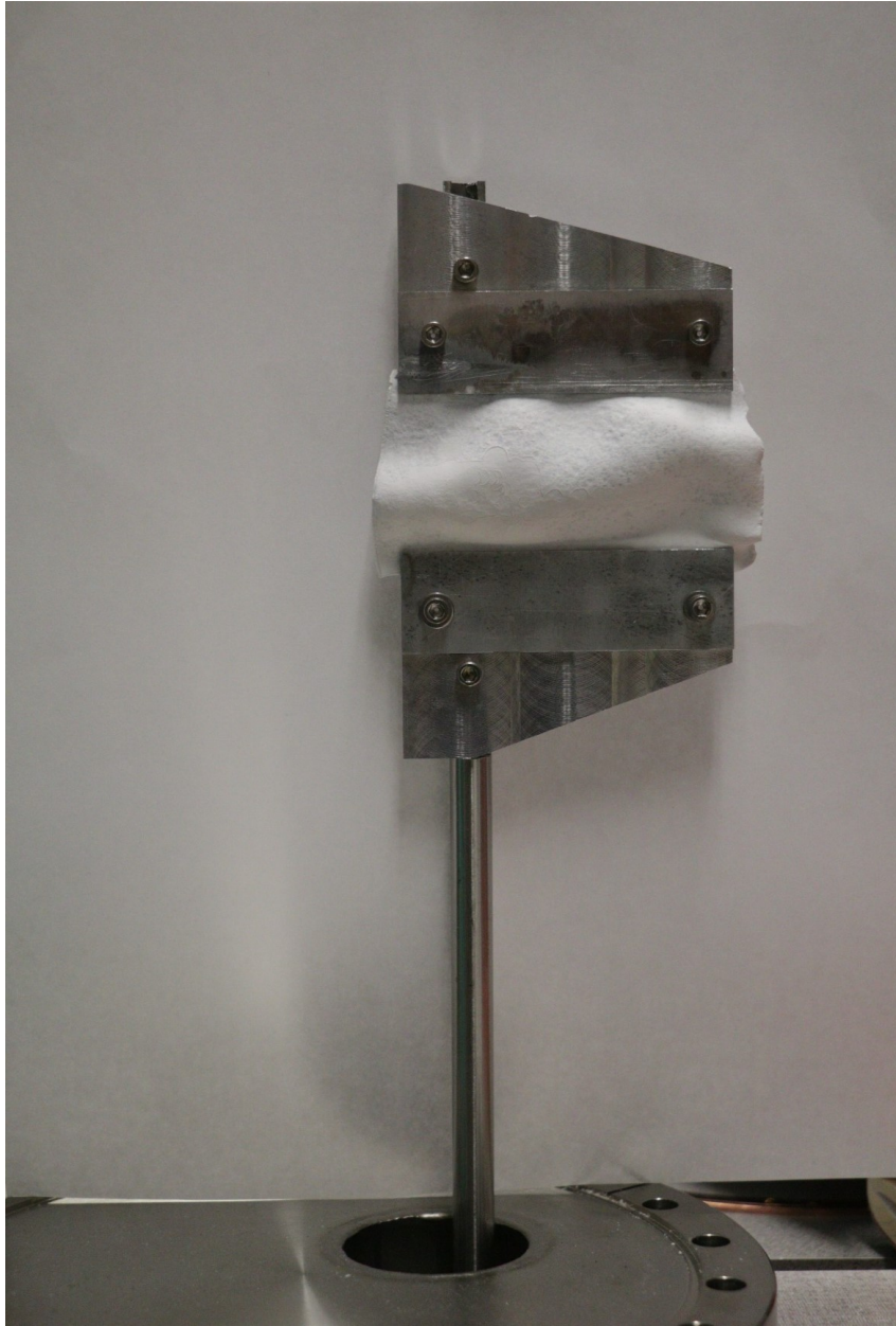
Figure 3.4: Ablation target taken out of vacuum. While in vacuum the target is composed of highly purified lithium although after removal from vacuum the target degrades over time and forms a white oxide layer as shown here.
