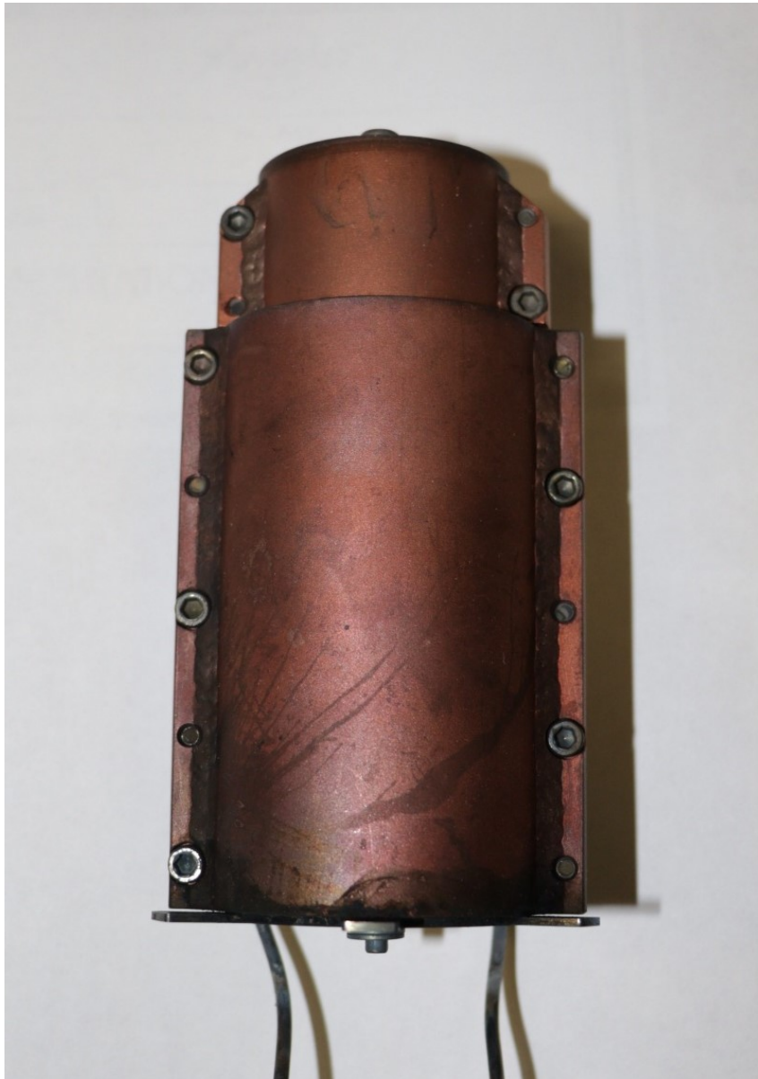
Figure 3.8: Directional oven taken out of vacuum. The two wires shown heat the reservoir and capillaries.
