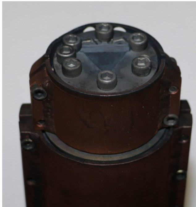
Figure 3.9: Close up of capillaries used to limit the divergence of the directional oven.
