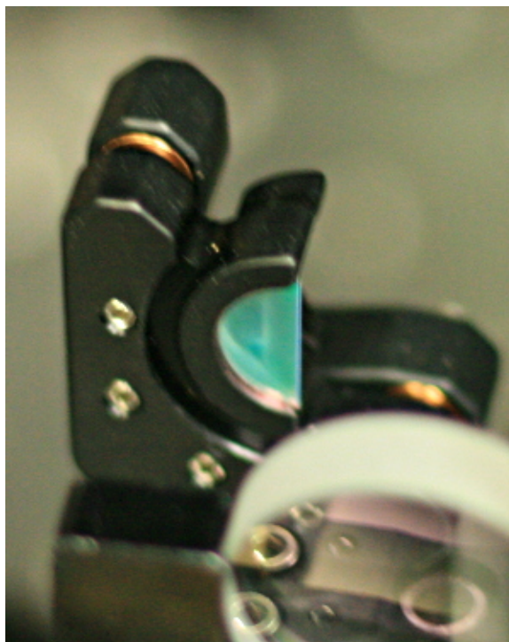
Figure 5.8: A D-shaped cut mirror (Thorlabs, BBD05-E03) is used to split the beam into equal halves at the equilibrium position of the particle. The mirror is mounted on a translation stage as it needs to be frequently aligned (§5.7).
