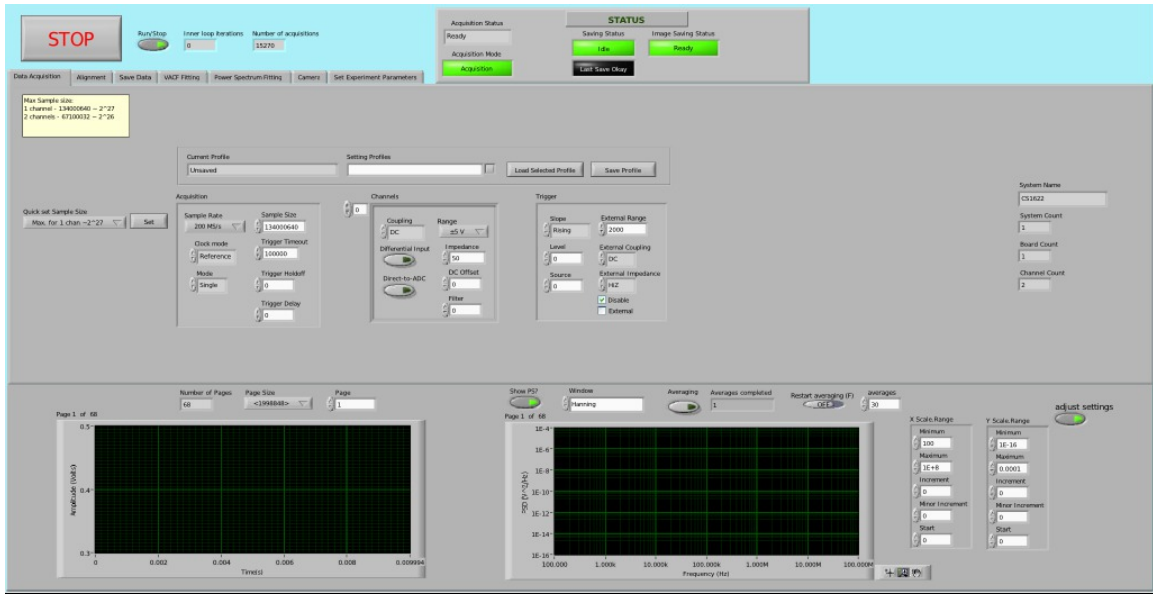
Figure 5.10: Main LabVIEW interface for data acquisition, alignment of cut mirror, and remote control of experimental parameters. The wave-form and power spectrum of a small segment of each acquisition is visualized at the bottom of the interface, and forms a very helpful tool to detect anomalies.
