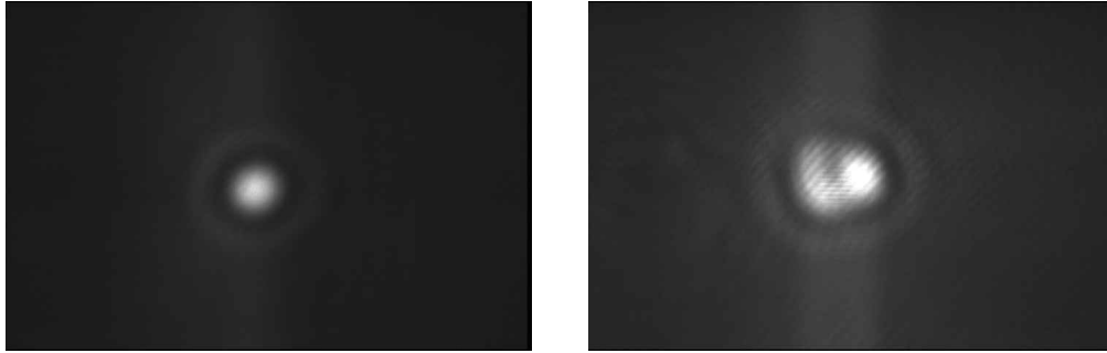
Figure 4.7: CCD images of trapped beads, formed using scattered light collected from the side of the trap. Left: A single 3.0 \mu\text{m} diameter microsphere; Right: multiple beads in the trap. The air pressure was 752 torr, and the trapping beam powers were 119 mW and 100 mW. Image courtesy of Tongcang Li.
