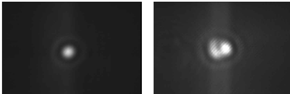
Figure 3.16: Left: A single optically trapped 3.0\text{-}\mu\text{m} diameter bead; Right: multiple (2 or maybe 3) optically trapped 3.0\text{-}\mu\text{m} beads. The air pressure is 752 torr. The powers of the two counter-propagating beams are 119 mW and 100 mW.
