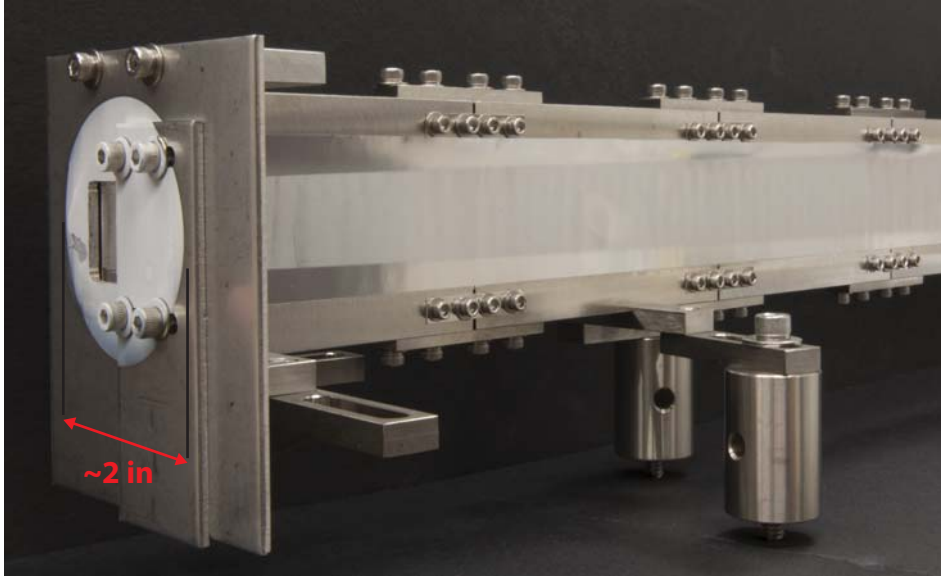
Figure 4.12: Lithium coating on magnet aperture (after removing magnets from chamber). The width of the coating on the magnet aperture was almost exactly the width that we had anticipated based on the apparatus geometry.
