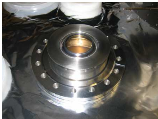
Figure 7.9: Photograph of the reentrant viewport. The size of the flange is nominally 6 in.
