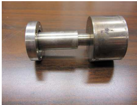
Figure 7.3: Lithium oven. The lithium is loaded into the reservoir which is heated to create an effusive beam of lithium atoms. Decreased wall thickness close to the reservoir (right) limits the heat flow from the reservoir to the rest of the vacuum chamber. The outer diameter of the reservoir is 1.5 in.
