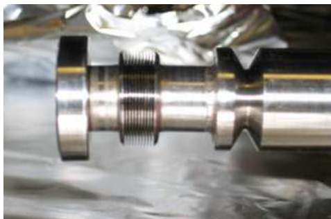
Figure 7.5: The small bellows at the end of the differential pumping tube allows for the alignment of the atomic beam axis between the oven chamber and the science chamber.
