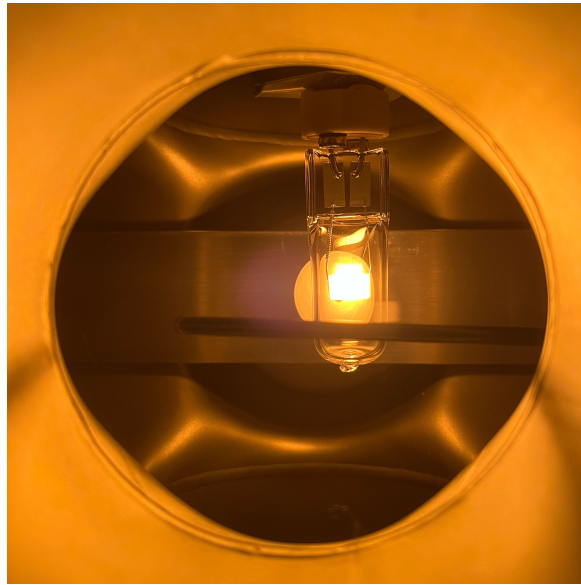
Figure 6.4: The graphene diaphragm in the cleaning chamber. The sample is heated up and cleaned by the radiation heat from the lamp.
